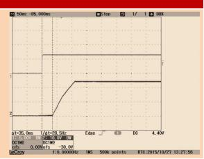
If the shutdown repeals the power supply starts with a delay of 35ms.
